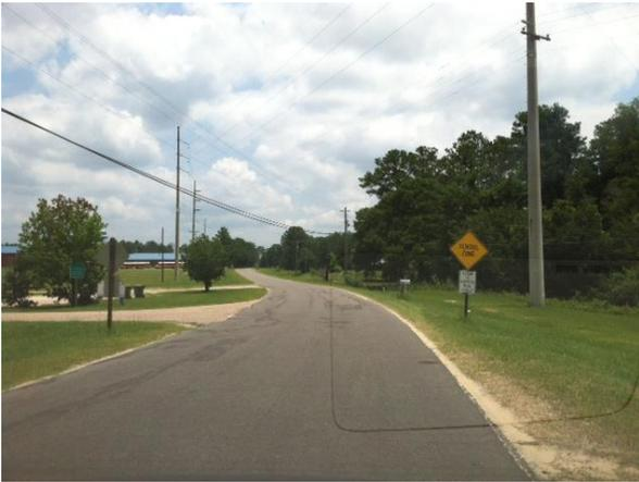
In addition to no sidewalks, the existing signage to let motorists know they are entering a school zone is extremely small and outdated. Signs should be large, have a posted speed limit, and have flashing lights. Signage should also be placed on the surrounding highways (GA Highways 27 and 82).
