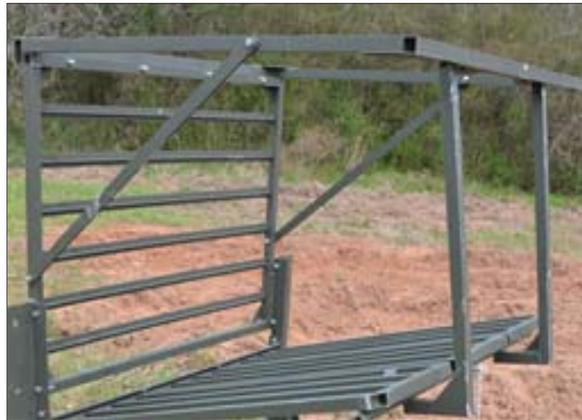
Figure 42: An example of an out-rigger used on a three panel rooter door. Photo Credit - MT Mengak, March 2014.
