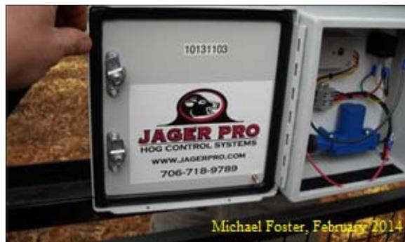
Figure 34: Jager Pro remote trigger control box.
